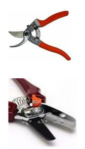
**Bypass secateurs:** These are the most common type, they work like a pair of scissors. They have one curved blade which cuts as it bypasses a curved jaw. They make a nice clean cut and are good for smaller stems. Some secateurs have a sap groove and others a wire cutter notch. Right and left hand versions are available.
